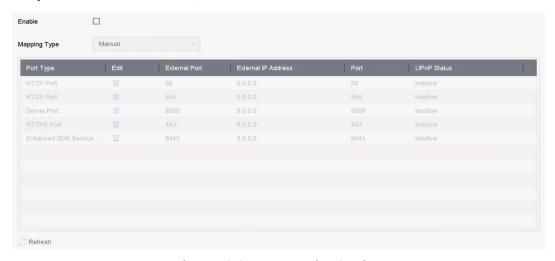
Figure 13-3 Port Mapping Setting
