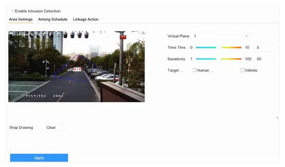
**Figure 6-6 Intrusion Detection**
