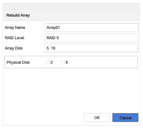
Figure 11-12 Rebuild Array
