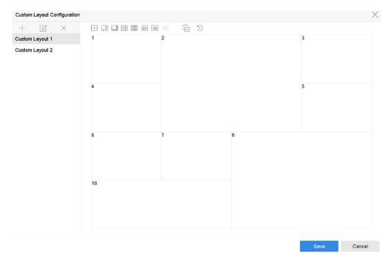
**Figure 3-3 Configure Live View Layout**
