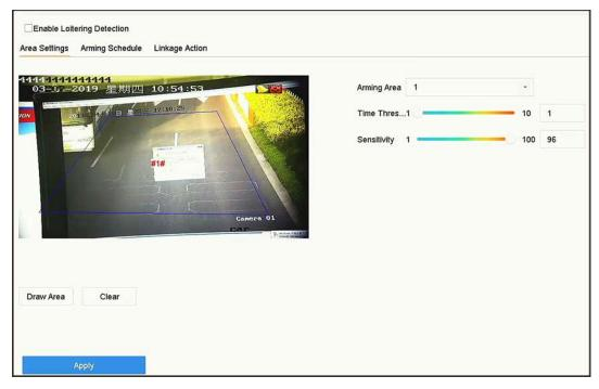
**Figure 6-9 Loitering Detection**
