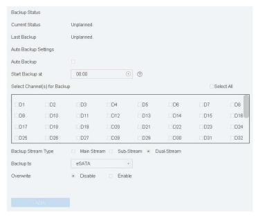
Figure 11-6 Configure eSATA for Auto Backup
