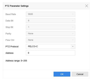
**Figure 3-7 PTZ Parameters Settings**
