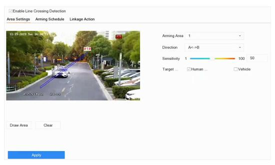
**Figure 6-5 Line Crossing Detection**
