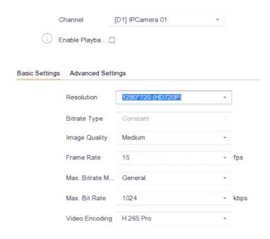
Figure 4-7 Transcoded Playback
