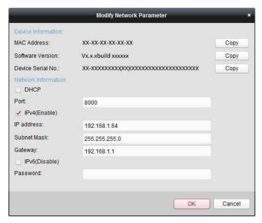
**Figure 1-6 Modify Network Parameters**
